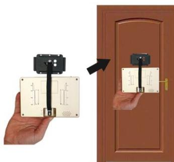
**04:** Insert the cable to the display according to the direction.
